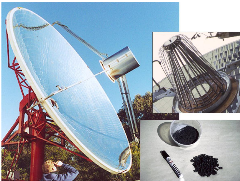
Figure 11: ANU's ammonia cracking receiver / reactor designed for operation at up to 30MPa 700°C.
