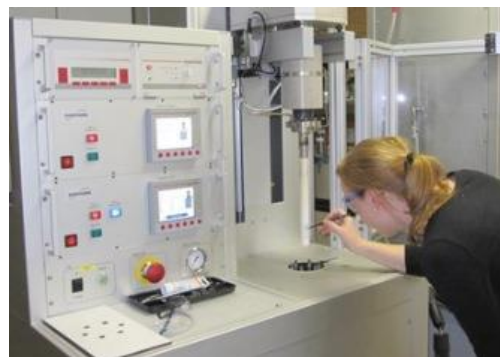
ABOVE: Joanne conducting high temperature gasification measurements at FZJ to determine the species evolved from Victorian brown coal
