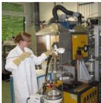
ABOVE: Joanne conducting high pressure measurements at KIT to determine fundamental kinetic parameters of VBC gasification.
