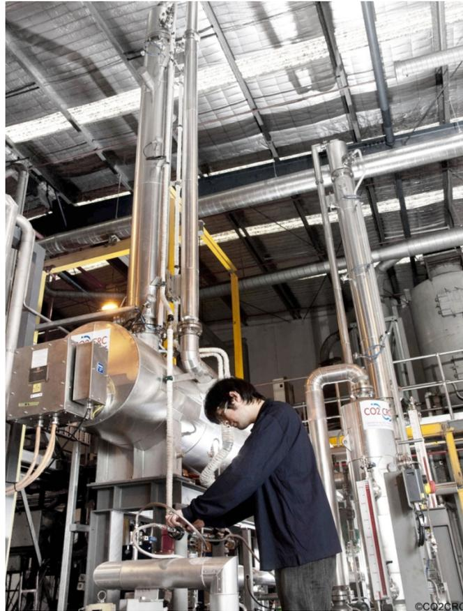
Figure 5.1.1 Solvent Absorption Capture Pilot Plant onsite at HRL Mulgrave
