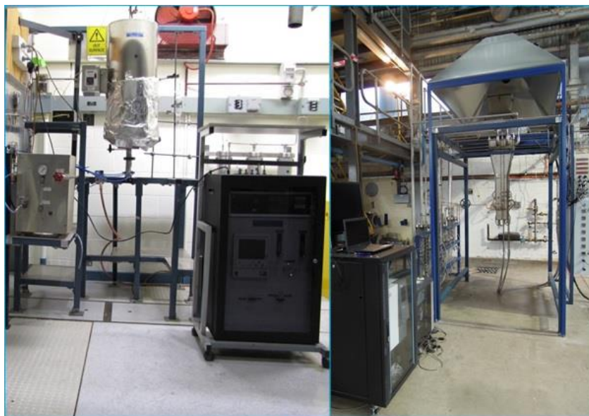
Figure 1: Chemical looping (a) bench scale system (Monash University) and (b) compact fully looped, continuously fed 10kW CLC reactor system (CSIRO).
