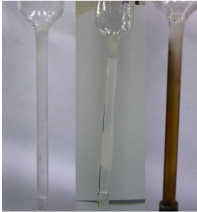
Figure 36 Tar at the outlet of the reactor after passing through a fixed-bed with and without catalyst.
