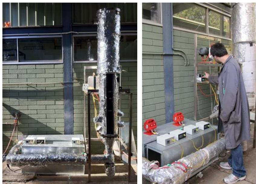
Figure 1: Continuous fluidised bed
