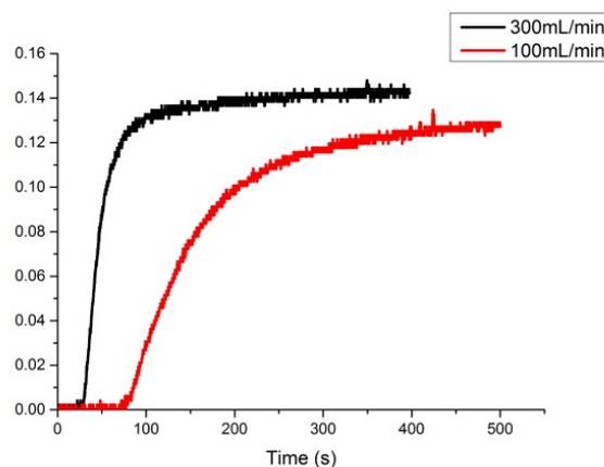
Figure 4. Breakthrough experiment with the brown coal monolith at room temperature and ambient pressure. The feed is 15% CO<sub>2</sub> in nitrogen.
