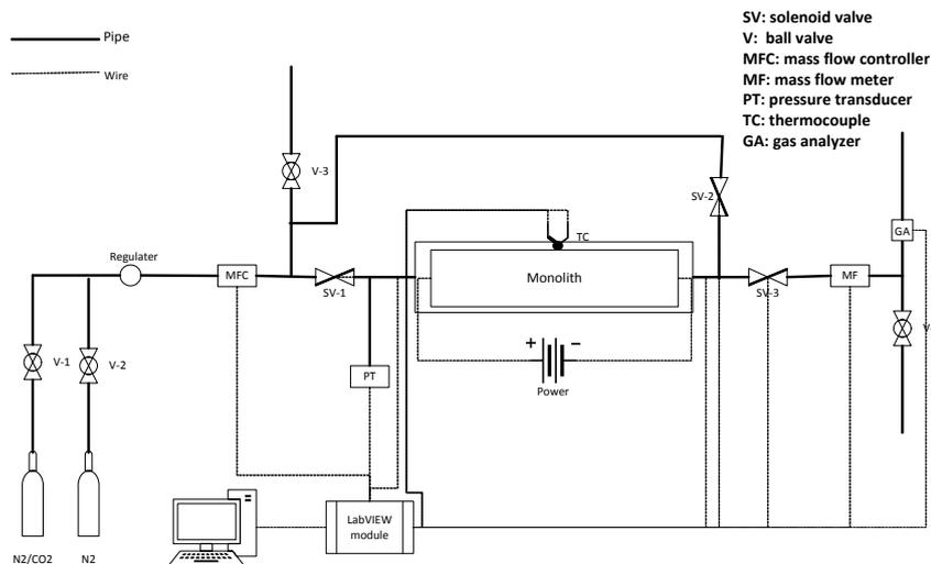
Fig. 3 Schematic of ESA apparatus
