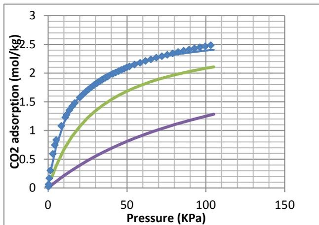
Fig. 2 Isotherms of CO<sub>2</sub> on brown coal monolith; symbol - experiment, lines – simulations
