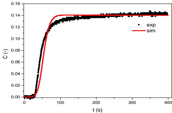
Fig. 5 Simulation of breakthrough at the flowrate of 300ml/min ( $K = 0.2 \text{ 1/s}$ )
