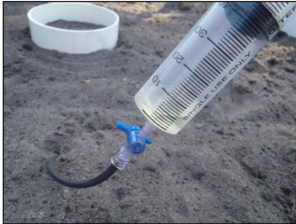
Figure 5.7 Retrieving the soil leachate through the LDPE extraction tube from the installed lysimeter.
