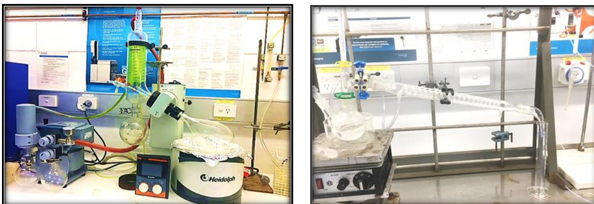
Fig.1: Apparatus for (a) vacuum, and (b) atmospheric distillation experiments
