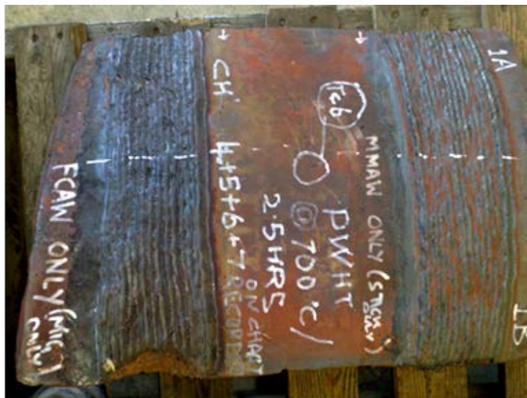
Figure 17 One of two CMV samples after completion of welding activity
