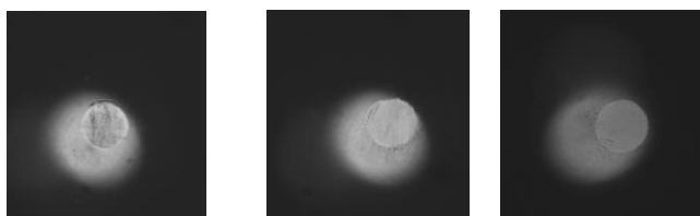
Wear scars from clean cylinder oil (left), and contaminated by brown MRC ash (centre), black MRC ash (right)
