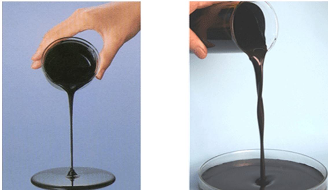
Figure 7 - Left, coal water fuel for a boiler by JGC; right, MRC for DICE
