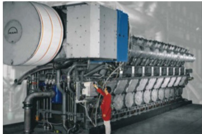
Figure 9 - A large medium speed engine by MAN (20 MW, 500 rpm)
