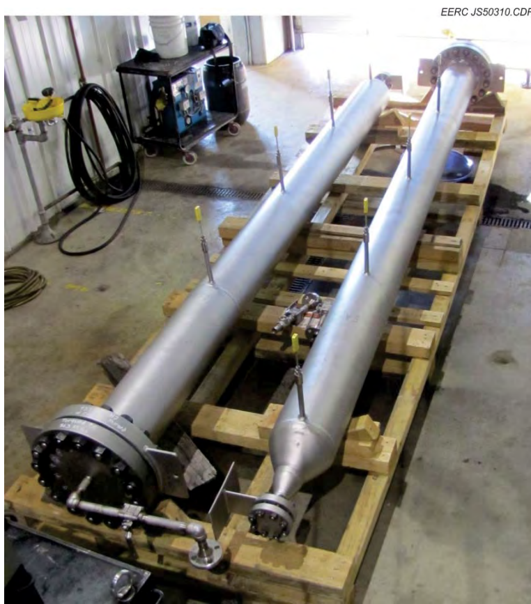
Figure 31. Sulfur capture fixed beds.
