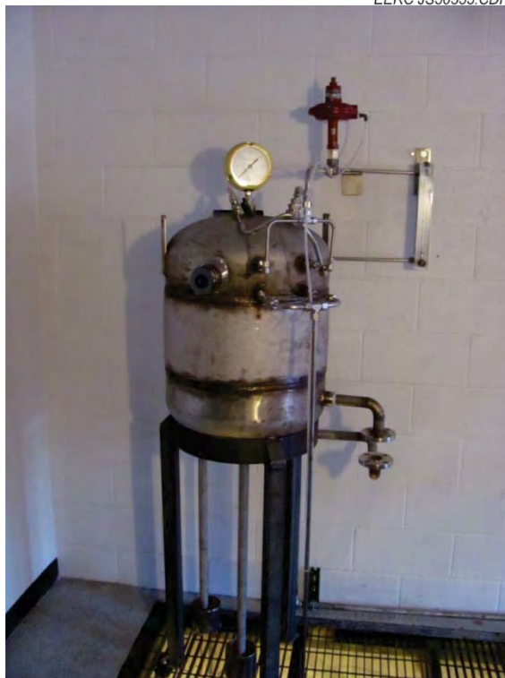
Figure 30. Dowtherm reservoir and cooling control valve.
